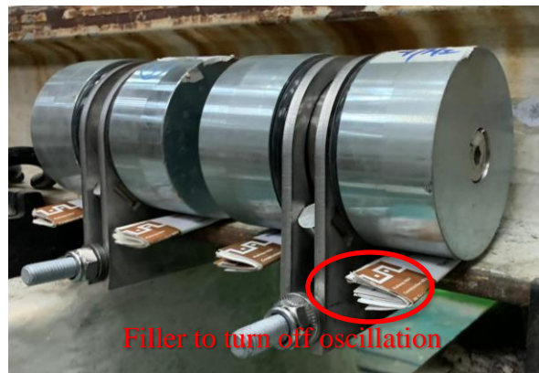
Figure 5: 2 sets of GBN STMD with in-phase oscillators
