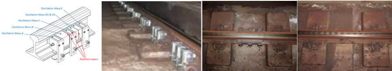
Fig. 8. 3D-views of the first-generation rail damper, photos of installed dampers and corrugation mark installed in 2010
